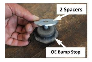
Note: The provided bump stop spacer must be installed as shown in order to insure proper travel and to avoid possible damage to shock if not properly installed.
