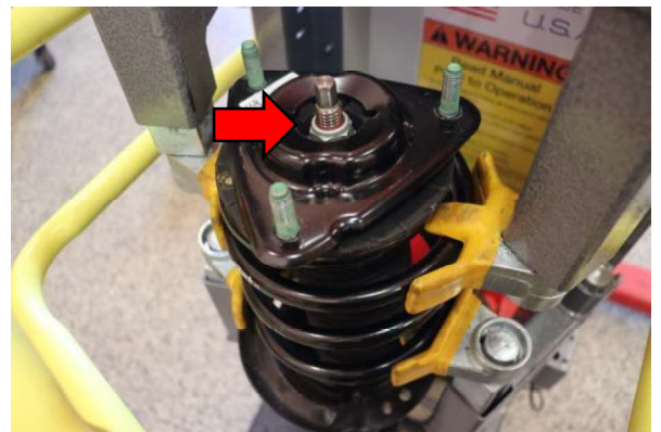
Step 18. Compress the Eibach spring. Install the OE top hat and bot assembly. Install the OE shock from below making sure the end of the spring aligns with the end of the lower spring isolator. Install and tighten 21mm shock shaft nut to factory specification.
