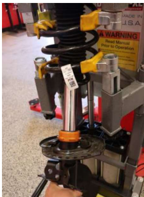
Step 17. Remove the shock from the compressed spring. Remove OE top hat and boot assembly. Decompress and remove OE spring from the spring compressor.
