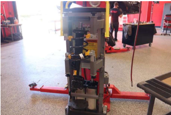
Step 15. Use a spring compressor to compress the shock assembly enough that the bottom of the spring is no longer contacting the lower spring perch.
