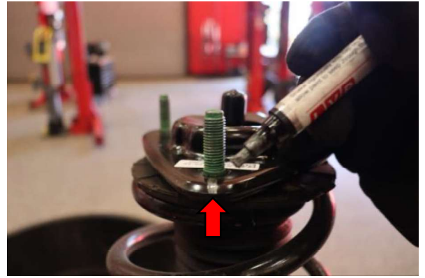
Step 14. Mark the shock assembly top hat to assist in alignment during reassembly.
