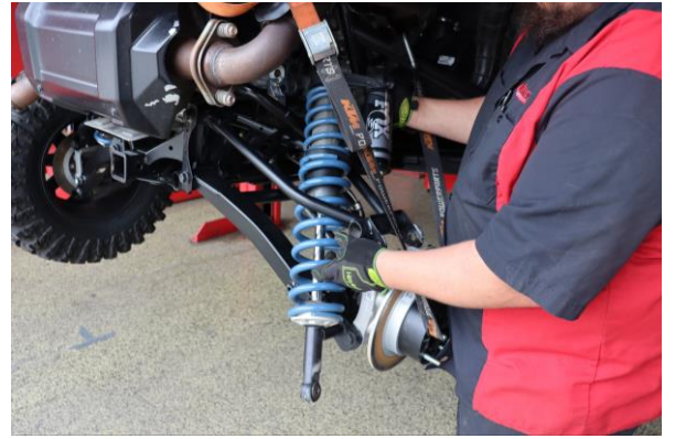
Step 8. Lift slightly on the wheel hub to remove the upper and lower shock mount bolts. Rotate the top of the shock out of the upper mount and lift out of the lower mount. Remove the shock assembly between the upper and lower control arm.
