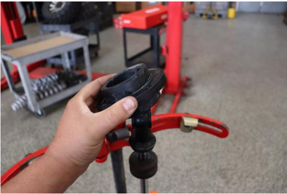
Step 9. Remove the OE spring slider.
