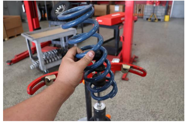
Step 8. Remove the OE main spring.
