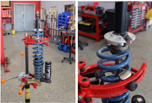
Step 9. Using a spring compressor, compress the shock assembly. Push the lower bump stop down enough that the lower spring retainer can clear the lower shock mount.
