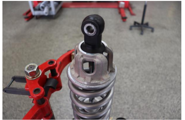
Step 16. Decompress assembly and ensure lower spring perch engages lower shock mount fully.
