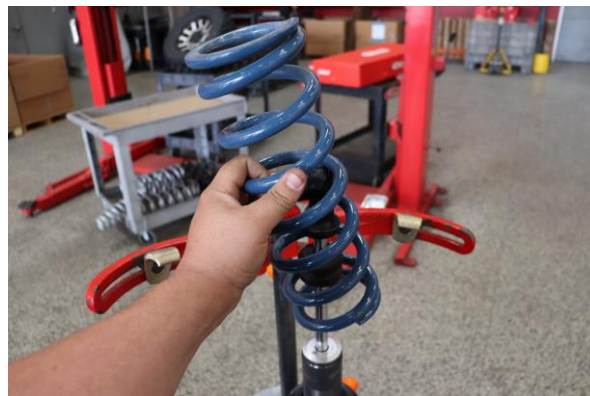
Step 8. Remove the OE main spring.
