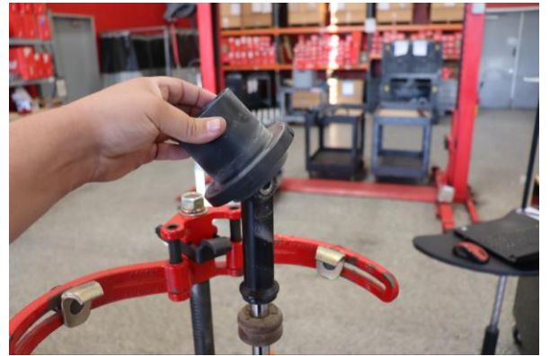
Step 16. Install spring slider.
