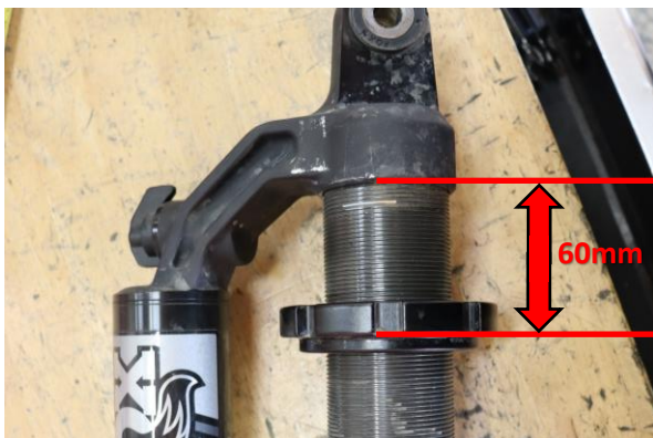
Step 11. Remove shock from the spring compressor. Adjust the upper spring perch to 60mm (2 23/64 in) measuring from the spring seat to the bottom of the bridge to set spring preload.
