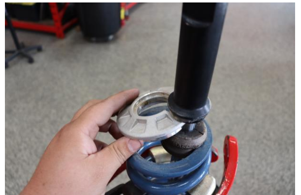
Step 18. Install the lower spring perch. Decompress the shock assembly and check to make sure the spring perch is fully engaged.
