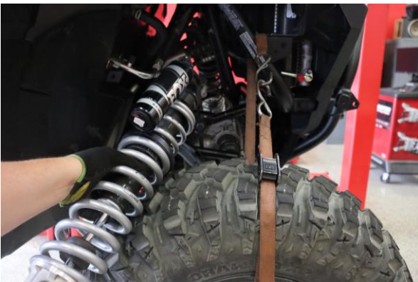
Step 17. Install shock assembly in the vehicle.
