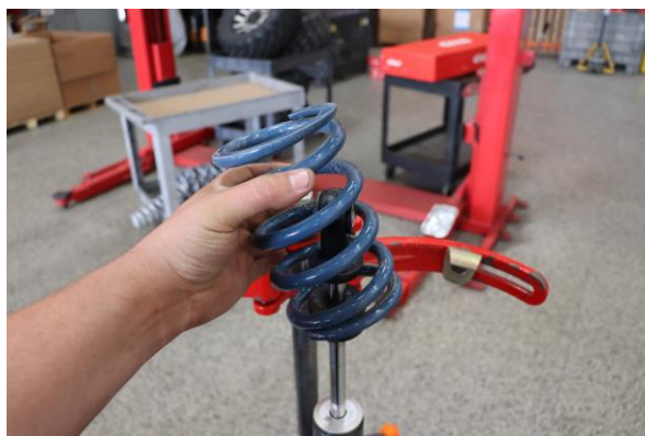
Step 10. Remove the OE tender spring
