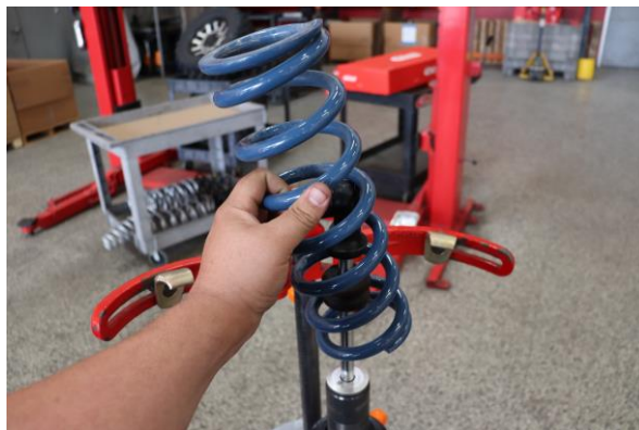
Step 8. Remove the OE main spring.
