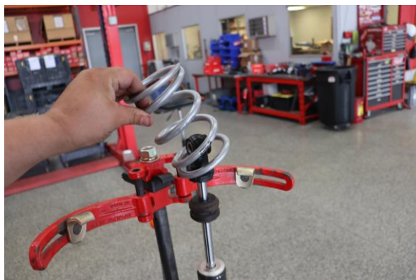
Step 12. Place shock back on the spring compressor. Install Eibach tender spring.
