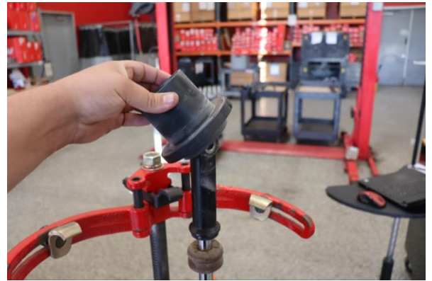
Step 16. Install spring slider.
