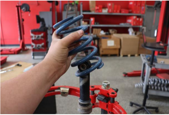
Step 13. Remove the OE tender spring.
